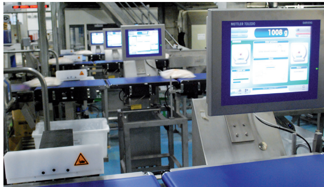
Versatile in-line checkweighers, perfectly adapted to the production line's requirements
